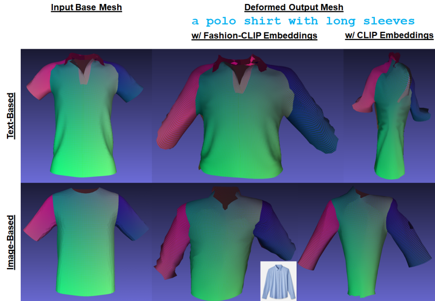
Fig. 8: Impact of the pre-trained CLIP on garment data: We disable all other supervisions and explore the impact of a pre-trained CLIP model on fashion data versus using the regular model to enforce embedding supervisions. We observe that regular CLIP embeddings result in distorted and unusable geometries regardless of whether the input is a text prompt or an image.
